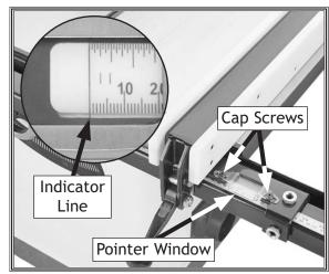
**Figure 22.** Fence pointer window alignment.
